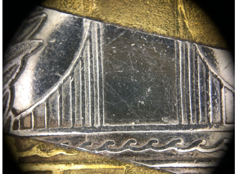
Close up of the embedded ferritic stainless-steel strip in NY630BC and NY630BD
