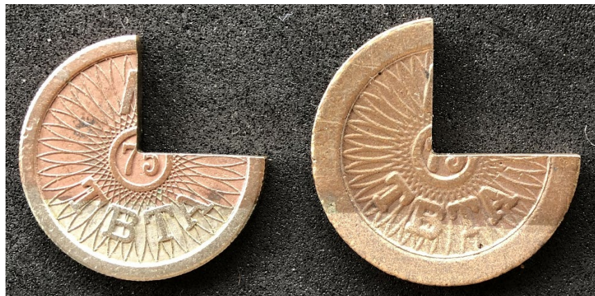
left: NY630AV – right: NY630AZ after 20 minutes in stripping solution
